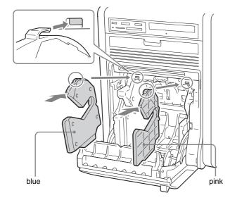
Press the portions indicated by the arrows until the tabs at the top lock into place.
